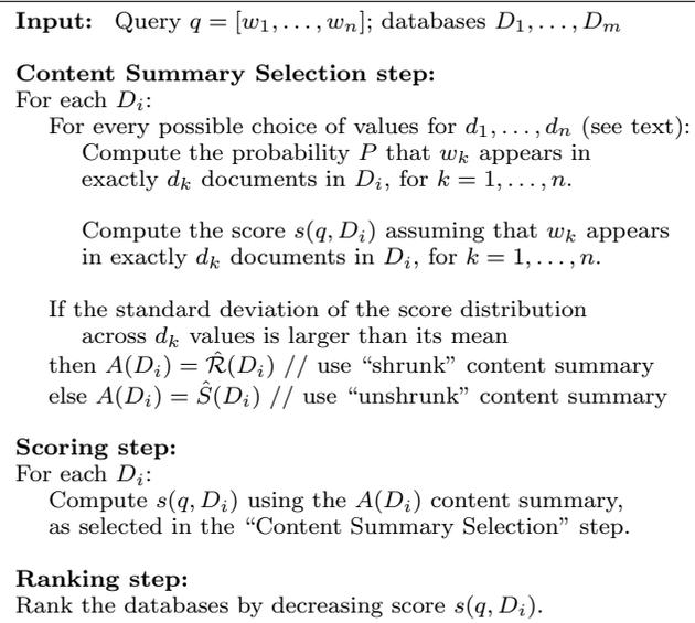
**Figure 3: Using shrinkage adaptively for database selection.**
